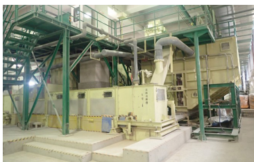
It is used as an aid to water removal from sewer slurry at the Tokyo Metropolitan Sewerage Service.
